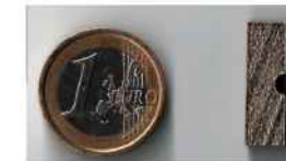
Fig. 2. Actual size (7 × 5 × 22 mm 3 ) of a CTOD resistance fatigue specimen.
