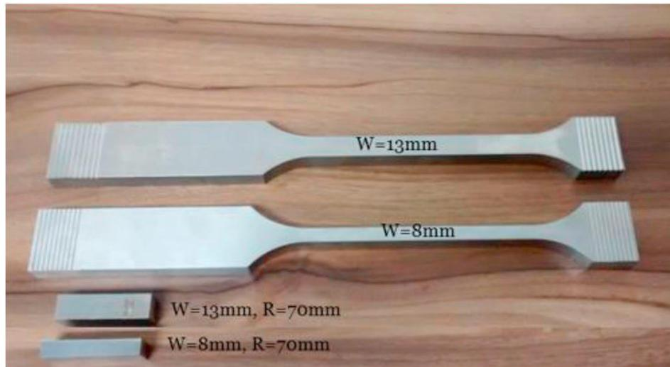
Figure 5-6 - Photograph of fretting fatigue specimens and pads. Both specimens and pads have the same height (13 mm).
