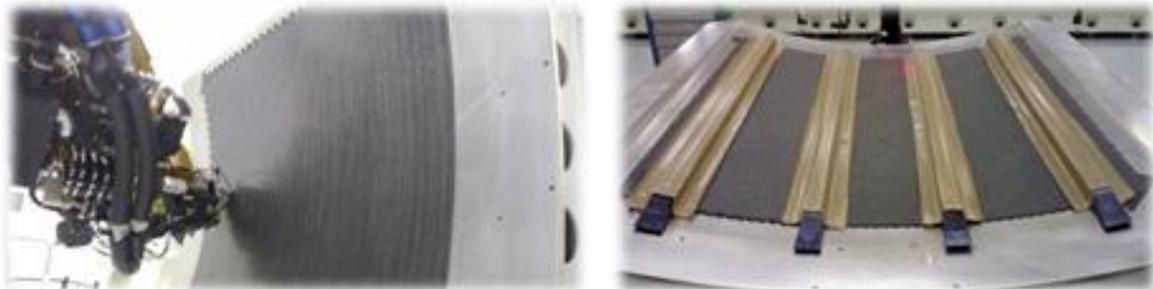
Figure 7-1 - Composite curved stiffened panel manufacturing.
