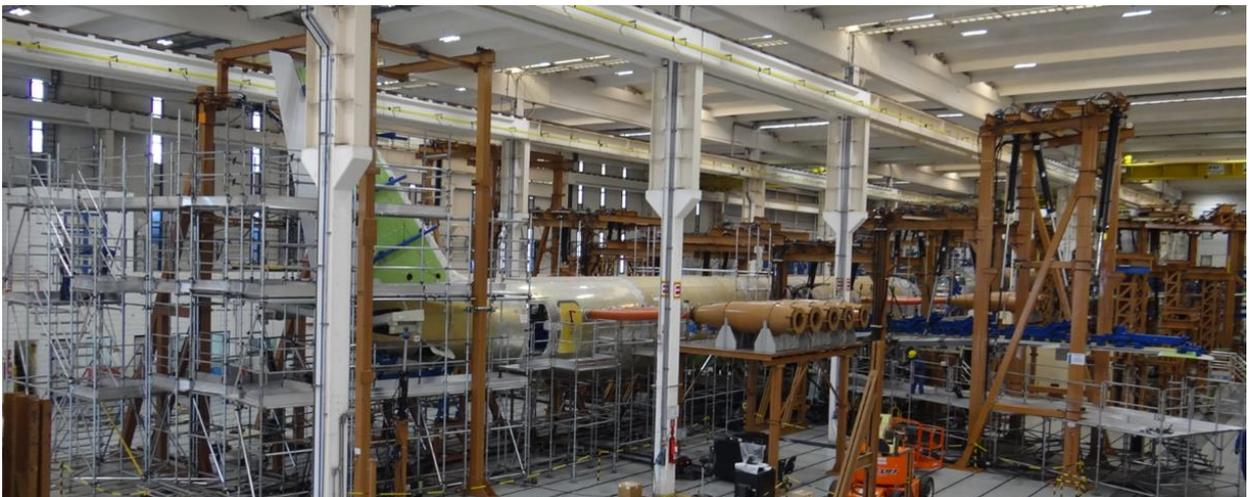
Figure 7-6 - Embraer 195 E2 (second generation) full-scale fatigue test overview.
