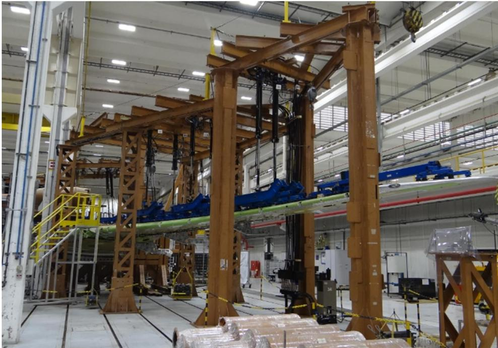
Figure 7-3 - Embraer 190 E2 (second generation) wing full-scale fatigue test overview.
