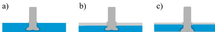
Figure 9-1 - Possible joint configurations of FricRiveting for multiple material types: a) metal-inserted, b) overlap, and c) sandwich-like joint.
