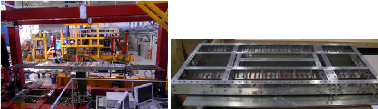
Figure 36. A simulated wing box comprised of composite upper and lower skin with aluminium spars and ribs
