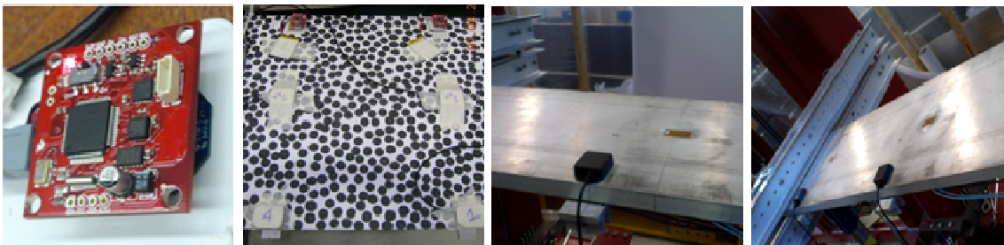
Figure 39. MEMS based load monitoring system under assessment
