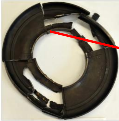
Figure 12. Remnants of the spacer after burst
