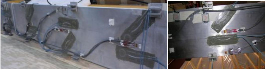
Figure 41. FBGs installed in the first SHM structural test bed, for point strain sensing
