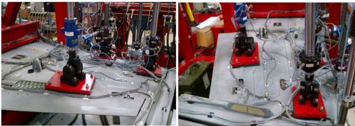
Figure 40. Optical fibre sensor for distributed sensing installed in the first SHM structural test bed
