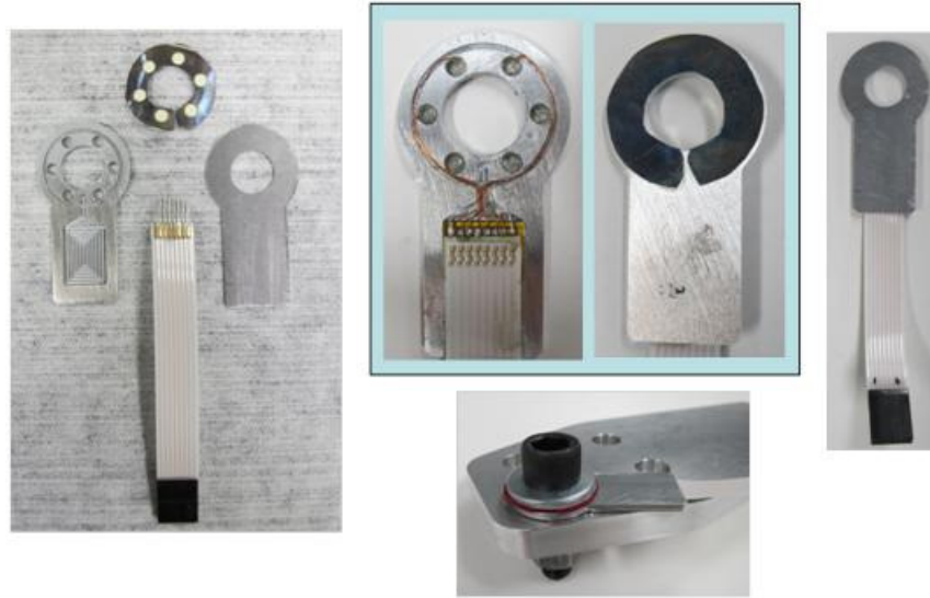
Figure 55. A trial version of the proposed sensor network (“Smart washer”) for SHM of fretting cracks
