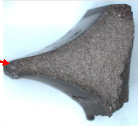
Figure 13. Microstructure analysis of the fragment of the burst spacer
