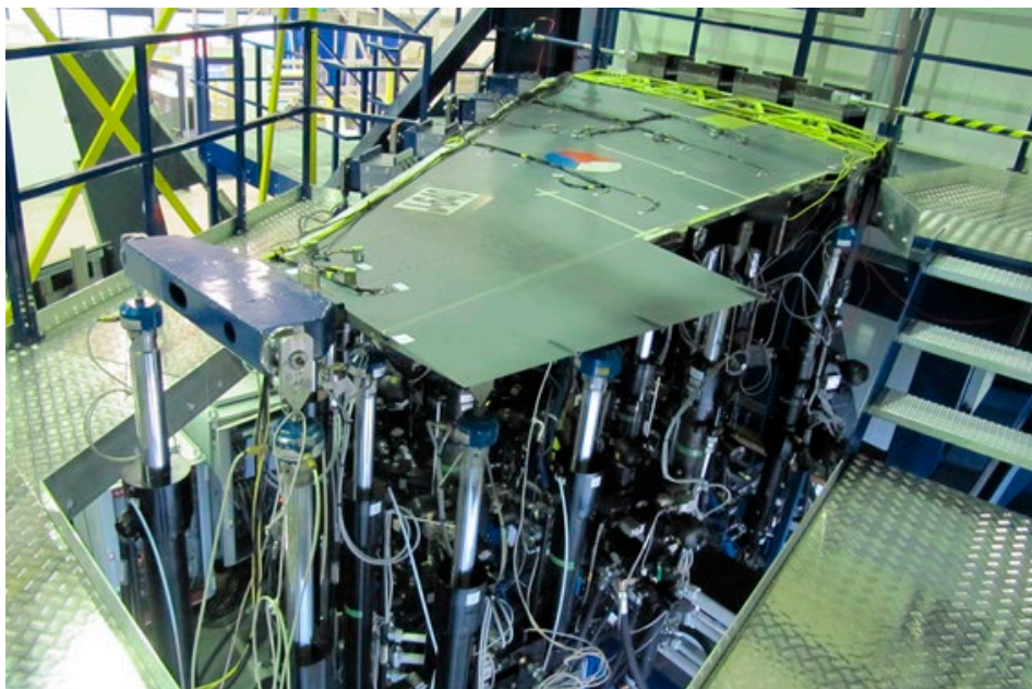
Figure 37: Impression of the F-16 wing test setup. Some of the acoustic emission sensors are visible in the foreground, at the wing tip.
