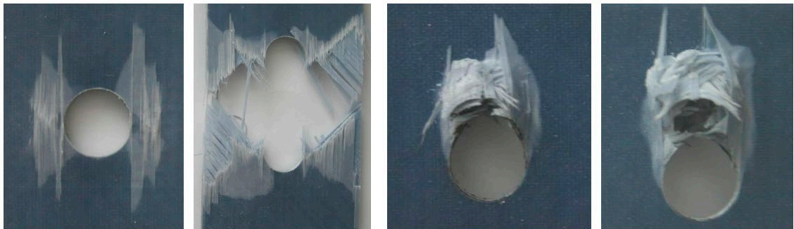
Typical open hole fatigue failure in glass fibre/epoxy
