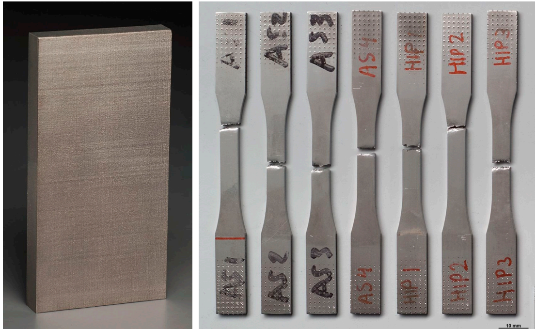
Figure 34: SLM specimen (left) and fatigue coupons (right) of Inconel 718.
