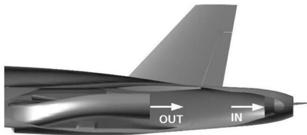
Fig. 15 Engine boundary values are defined at the compressor location and at the nozzle inflow location.
