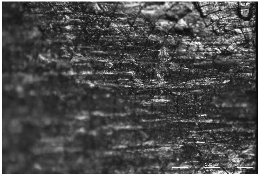
Fig. 47 Markerband III 2R-CA-4 fracture surface
