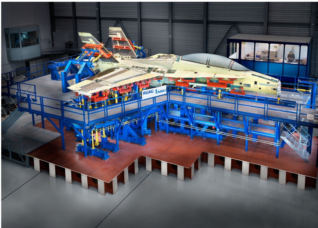
Fig. 38 Swiss F/A-18 Full Scale Fatigue Test
