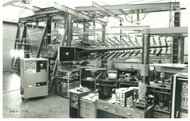
Fig. 37 Venom DH-112 test set up
