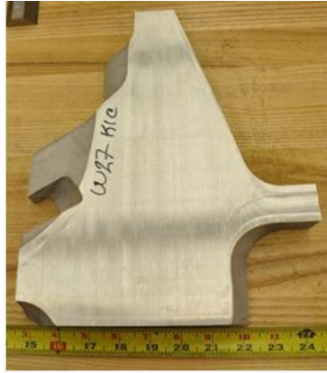
MSI ends are squared and specimen slices are cut.
