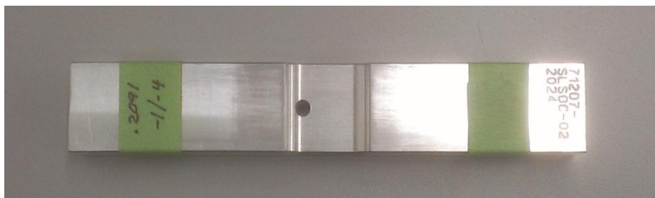
Figure 9.6-50. Pre-Test Open Hole Fatigue Test Specimen
