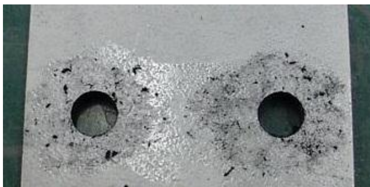
Figure 9.11-62. Interface Burrs and Surface Contamination in Carbon Fiber-Reinforced Composite-Metal Joint
