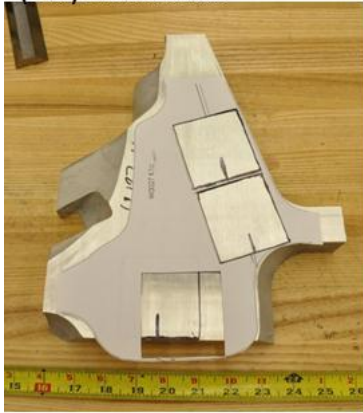
The specimens are cut out from the print-off.
