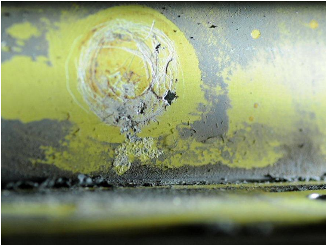
Figure 9.11-32. Wing Aft Spar Corrosion
