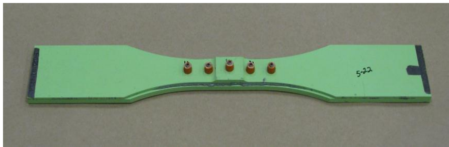
Figure 9.6-49. Pre-Test Joint Fatigue Test Specimen
