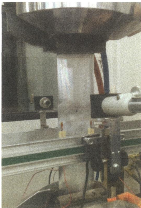
Figure 9.6-60. SOLR Specimen (Plate with Center Hole) Mounted in Servo-Hydraulic Test Machine
