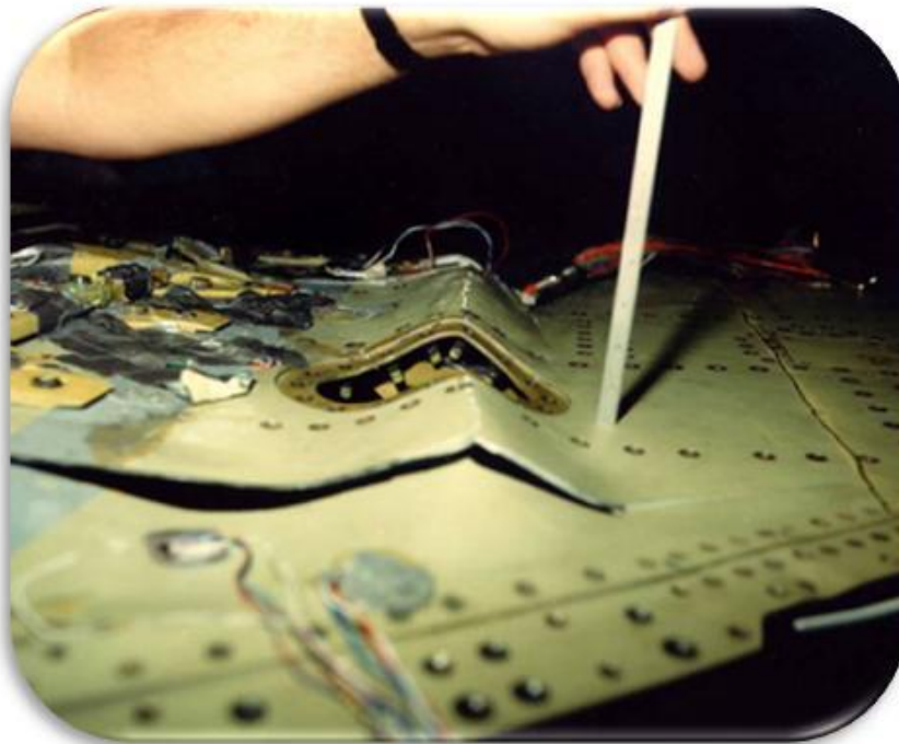
Figure 9.7-20. F-16C Block 30 Wing Failure at 128% DLL
