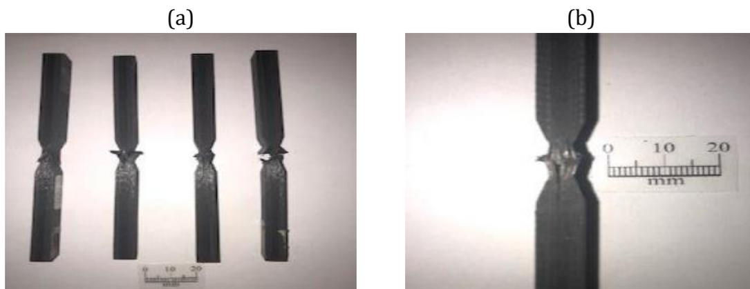
Figure 44 - (a) Coupons after the fatigue tests and (b) detail of the failure mode obtained in a sample coupon.
