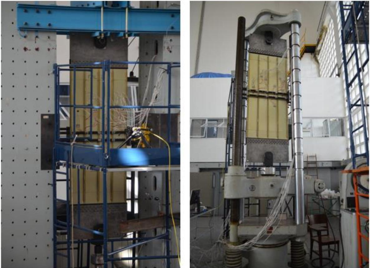
Figure 28 - Experimental test setup for fatigue tests (left) and residual strength tests (right).
