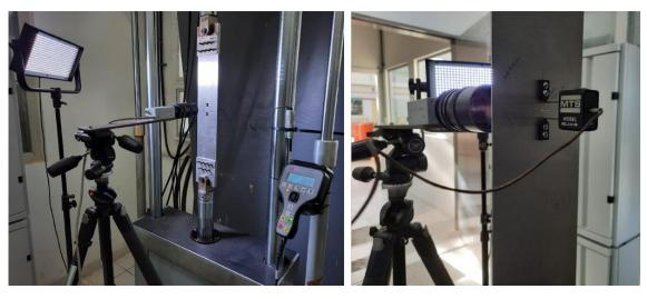
Figure 6 - Test machine with specimen and instrumentation installed.
