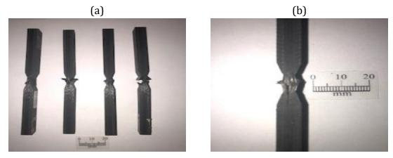
Figure 44 - (a) Coupons after the fatigue tests and (b) detail of the failure mode obtained in a sample coupon.
