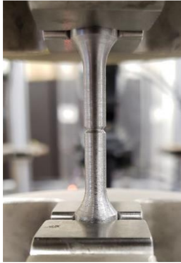
Figure 18: Experimental setup of notched AISI 4340 fatigue coupons
