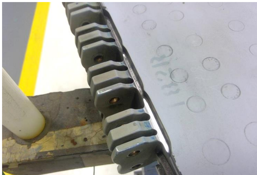
Figure 7: Light repair blend
