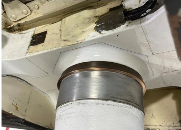
Figure 11: Bushing material build up repair with cadmium plating
