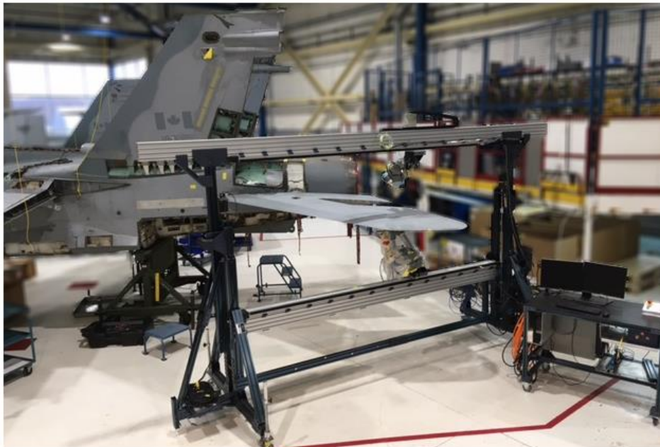
Figure 27: Robotized ultrasonic phased array C-Scan arrangement
