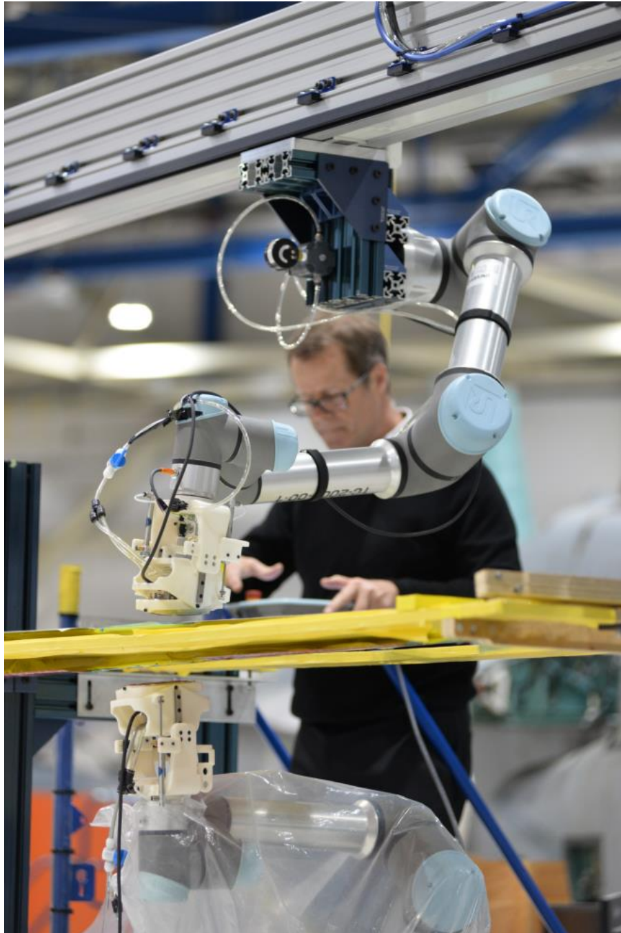
Figure 28: Robotized ultrasonic phased array C-Scan sensors
