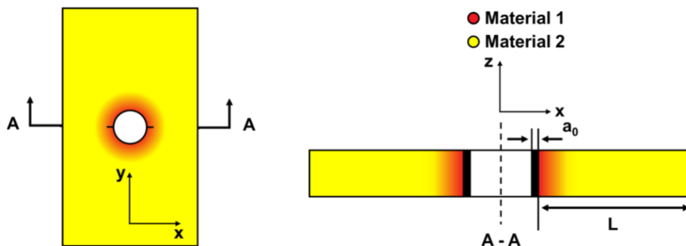
Figure 53: Custom graded specimen with potential function
