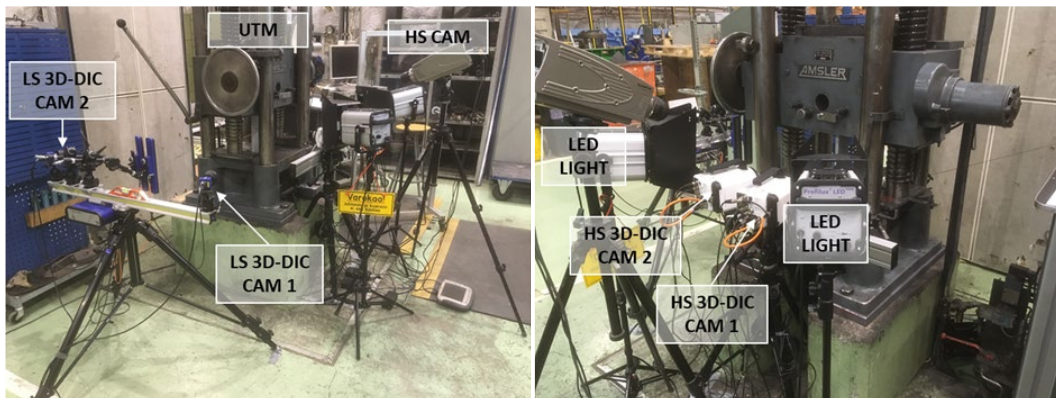
Figure 60: Test arrangements for the IWSLJ coupon static tests [107]. HS = high-speed camera, LS = low-speed camera. Figure courtesy of VTT.
