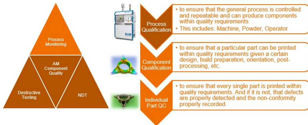
Figure 35: Stages of additive manufacturing quality assurance and control and supporting methods for these. Figure courtesy of VTT.
