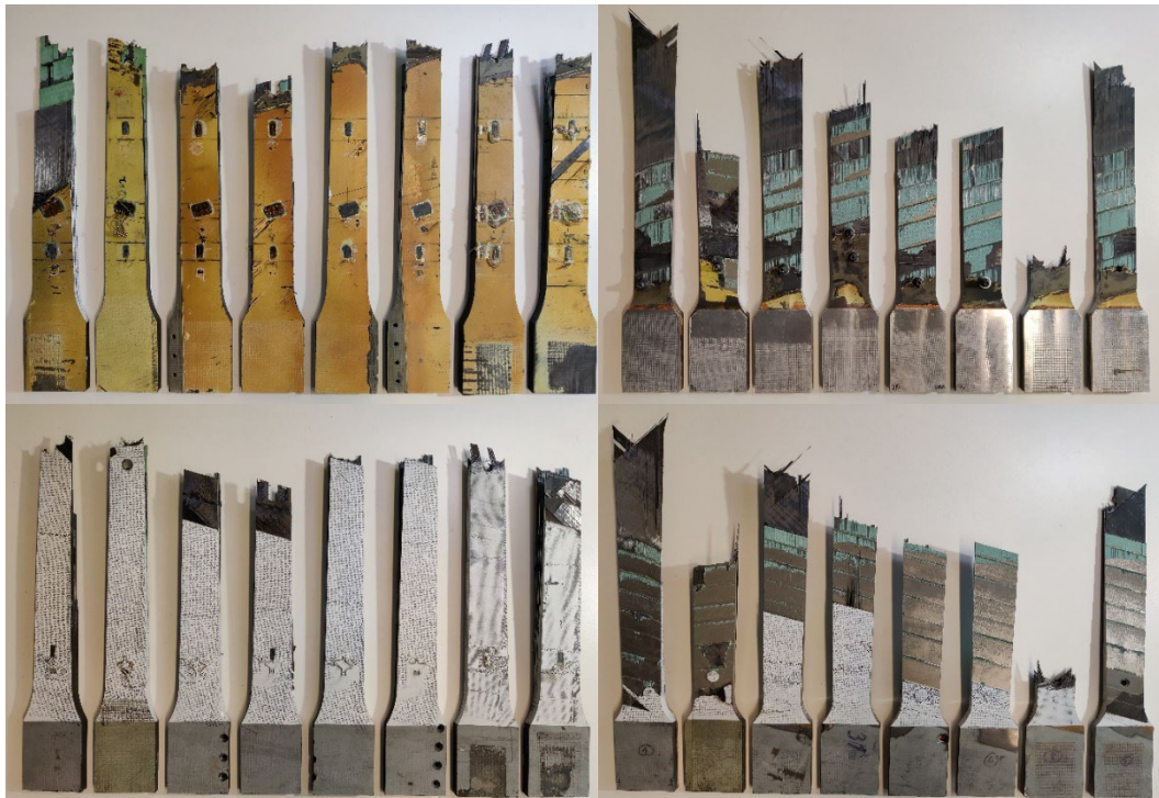
Figure 61: Failed specimen, static tests, IML side (upper), OML side (lower) [107]. Figure courtesy of VTT.
