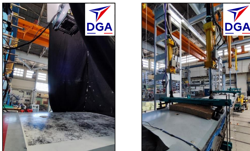
Figure 2: Left : Example of DIC placed on an area of interest on the wing. Right: Wing extrados and gauges wires
