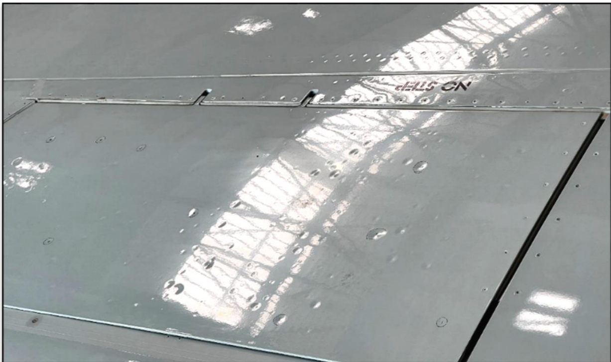
Figure 1: Hail damage on an aircraft wing
