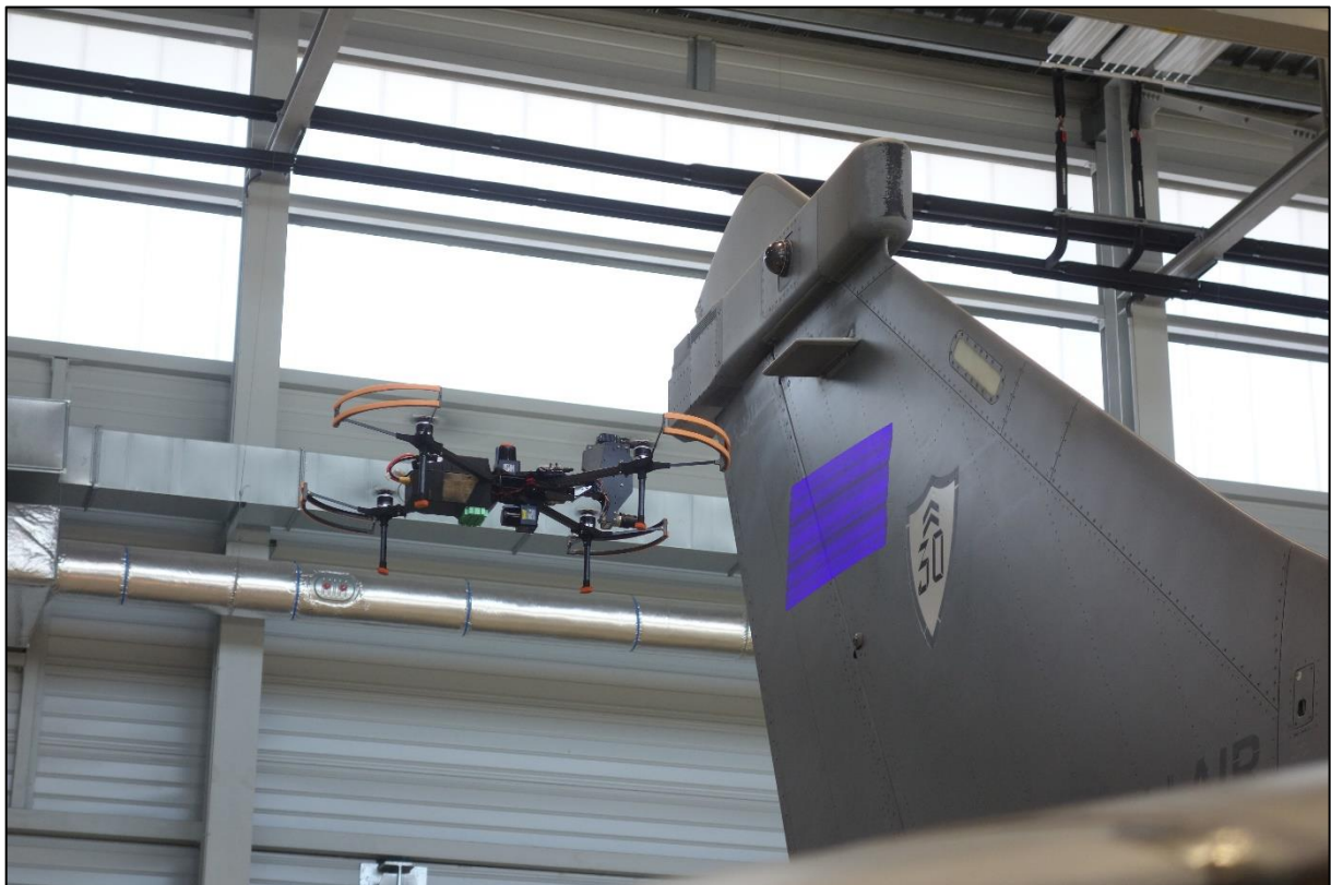
Figure 3: Iris dentCHECK inspection on Rafale Fighter aircraft
