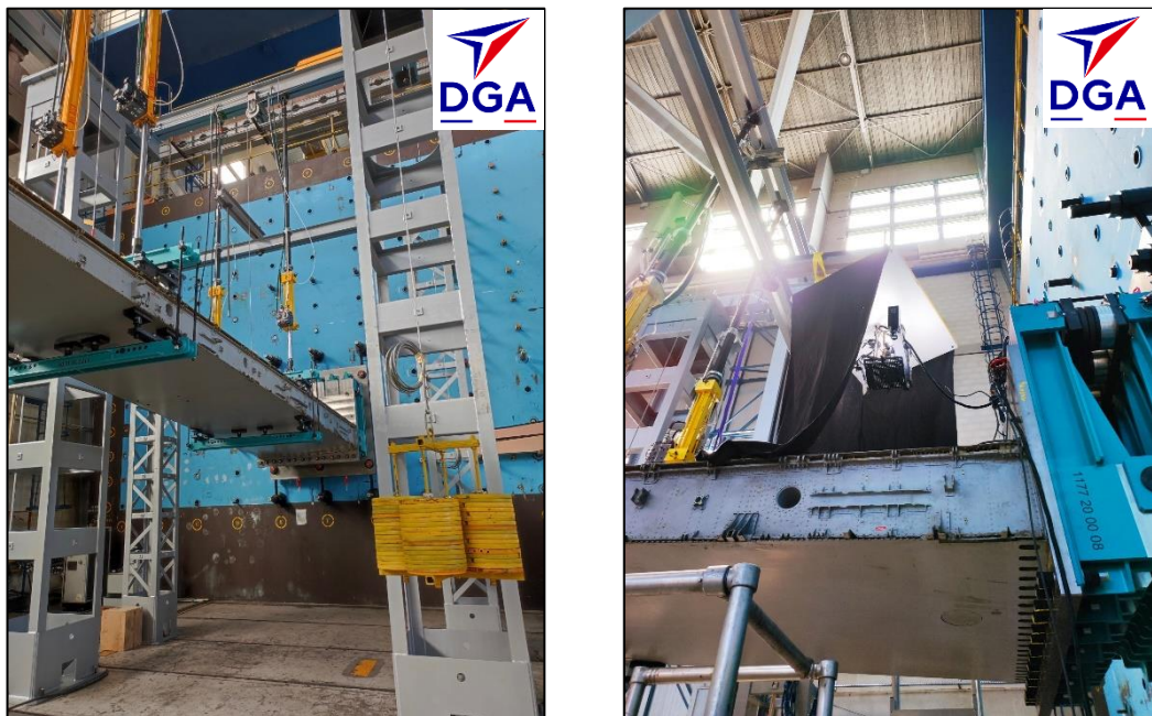
Figure 3: Test setting. Left : overall view, Right : DIC setup including darkroom preventing parasite reflections from the outside
