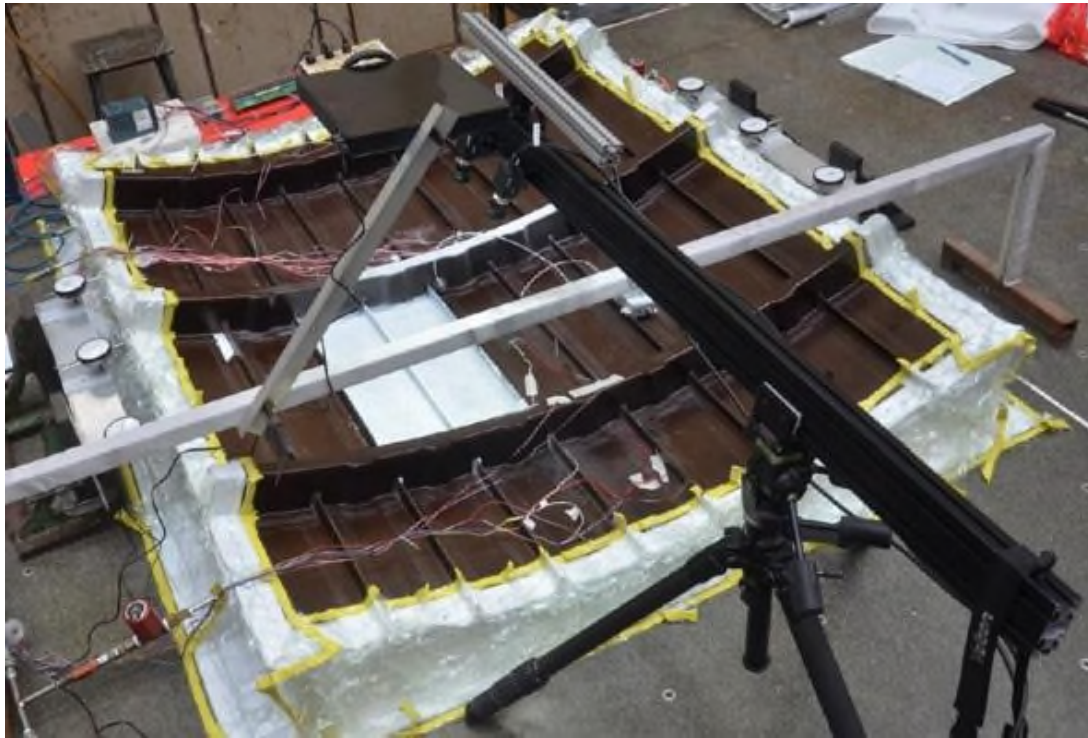
Figure 6: Test set up of a fuselage panel tested by Vacuum Test
