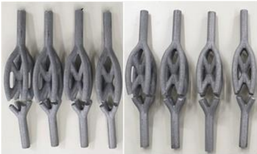
Figure 25: Fatigue test specimens and
