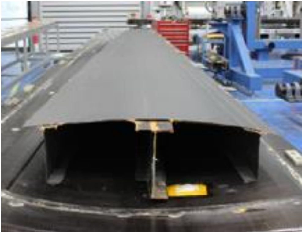
Figure 21: Final demonstrator integral wing-box infused component
