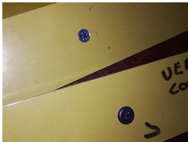
Figure 4.1 Bolted lap shear specimens (Flat and flush head Hi-Loks were used).
