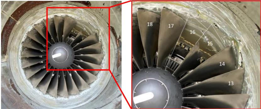
Figure 5.4.1 Fractured Fan blades
