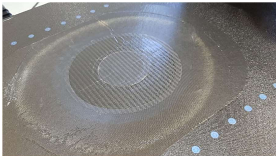
Figure 4.c: Final repaired panel.
