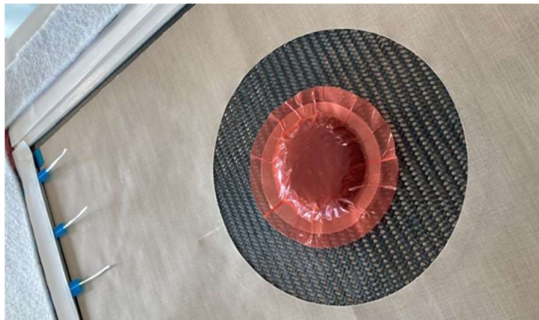
Figure 4.a: Repair layout with the new method
