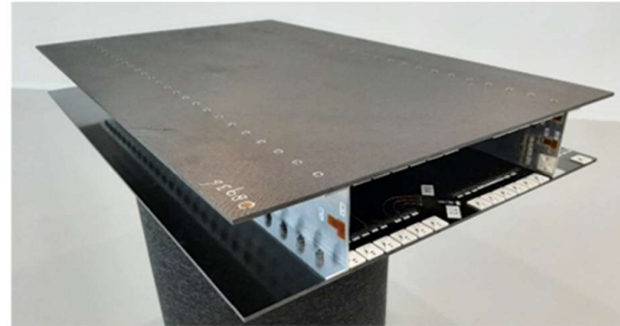
Figure 5.b: Assembled wing box.
