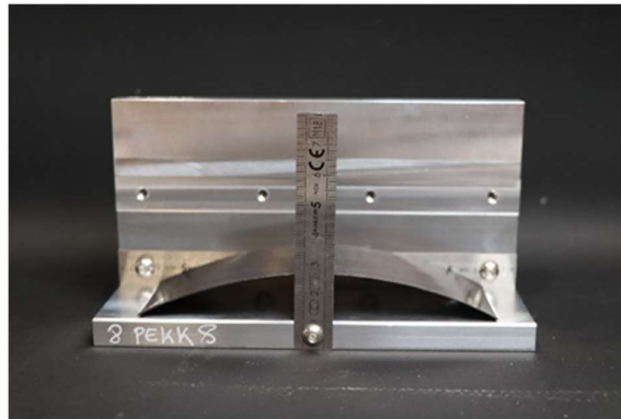
Figure 13 Measurement of the curvature of a cross-ply after one of the long cycles.
