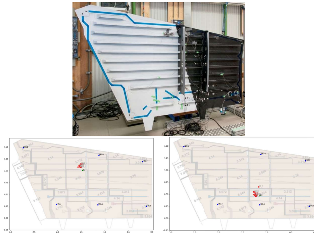
Figure 19 Impact localisation with FBGs on a stiffened thermoplastic horizontal tail plane.
