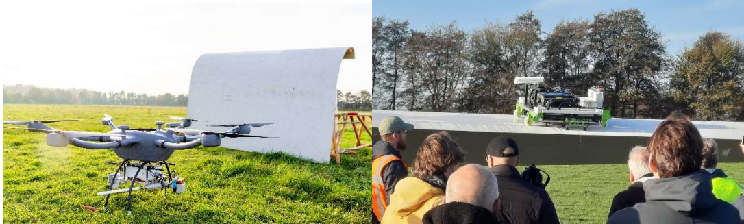
Figure 17 Final demonstration of AIRTuB program. Left: drone equipped with a miniaturized laser line scanner. Right: ultrasonic inspection performed with a crawler.
