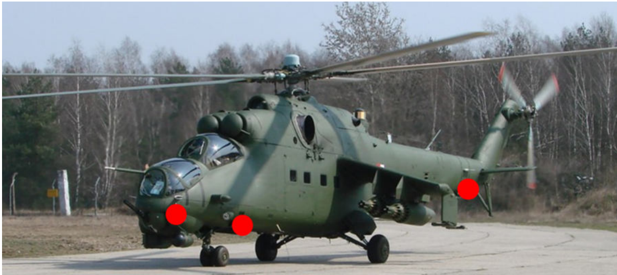
Figure 2. Location of sensors on the airframe of the Mi-24 helicopter
