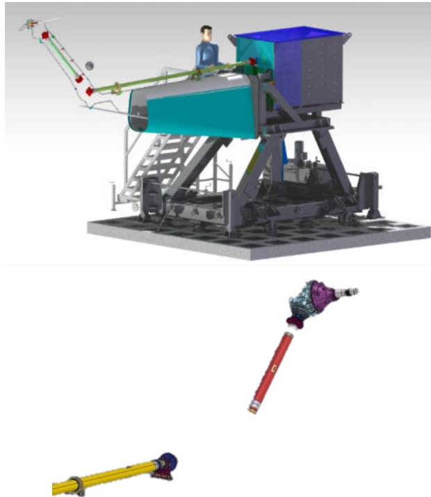
Figure 2. Ground test stand for impact detection and the region of interest
