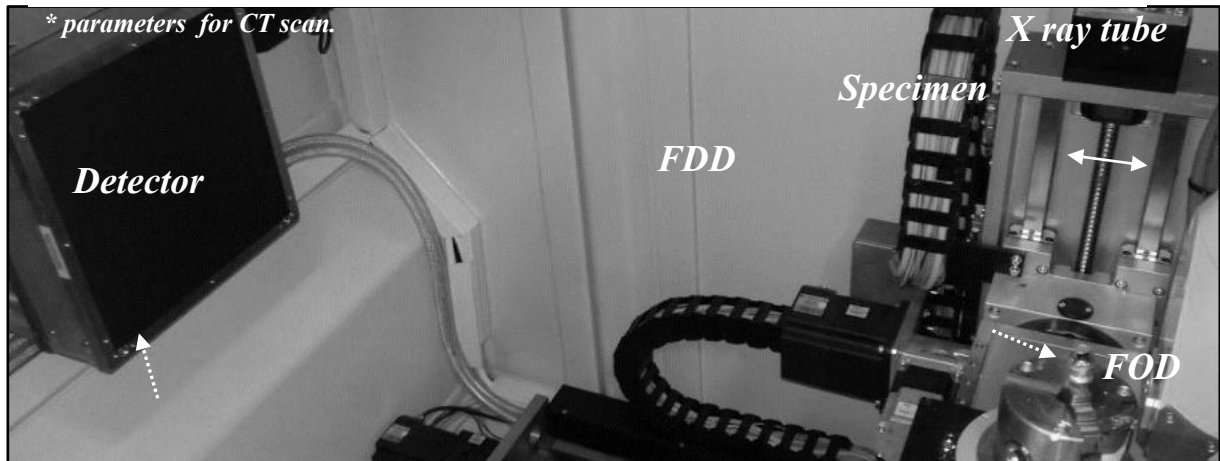
Fig. 3. CT System with parameters used for tested specimens.
