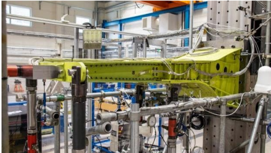
Figure 2.1-6. The test object and arrangement of the wing-to-fuselage joint test.
