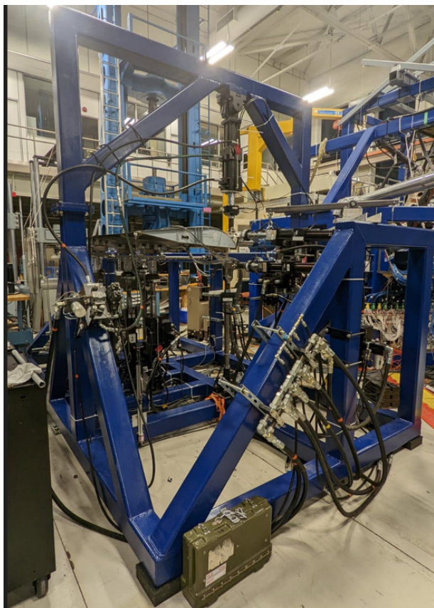
Figure 24: FTS4 – F/A-18 Trailing Edge Flap Component Test Rig
