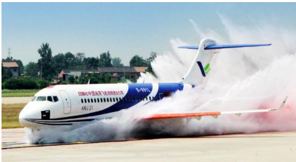
Figure 1: Spray of C909 aircraft taxiing on the water runway
