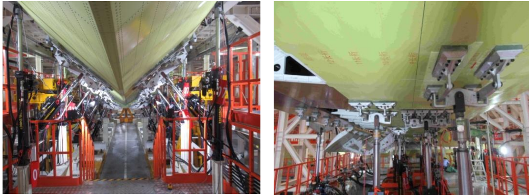
Figure 141: Fatigue Test Loading System
