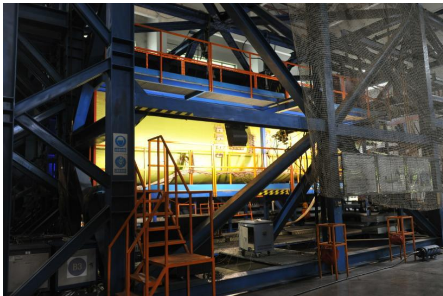
Figure 97: MA600F Fuselage Structure Full Scale Fatigue Test
