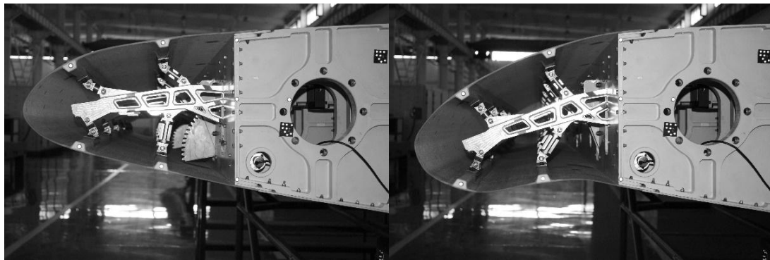
Figure 107: Comparison of the profiles before and after drooping
