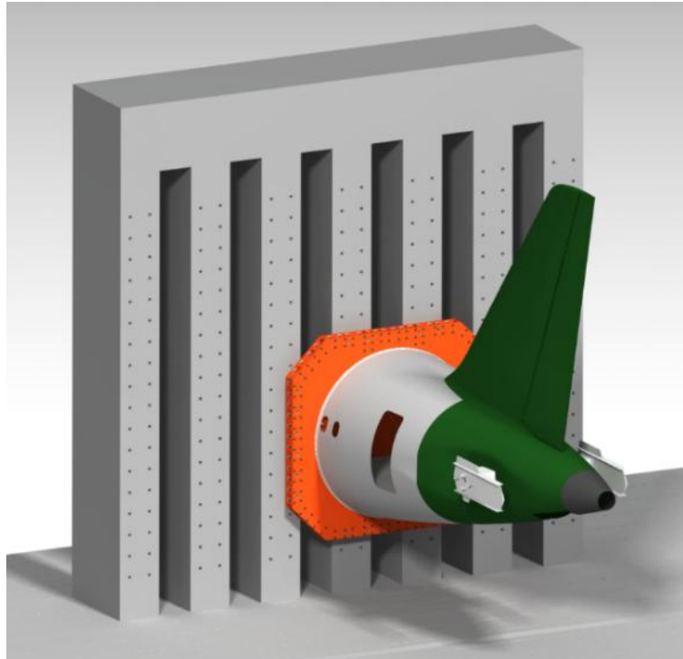
Figure 143: Schematic diagram of test specimen and constraint form
