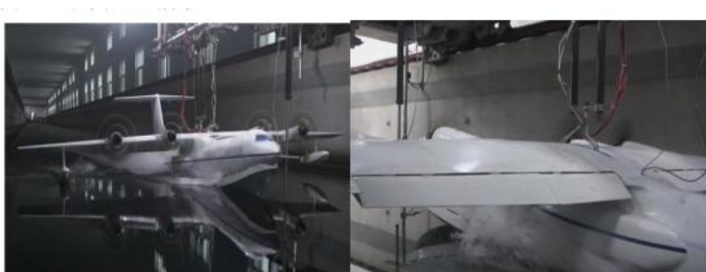
Figure 151: Full aircraft model splash test
