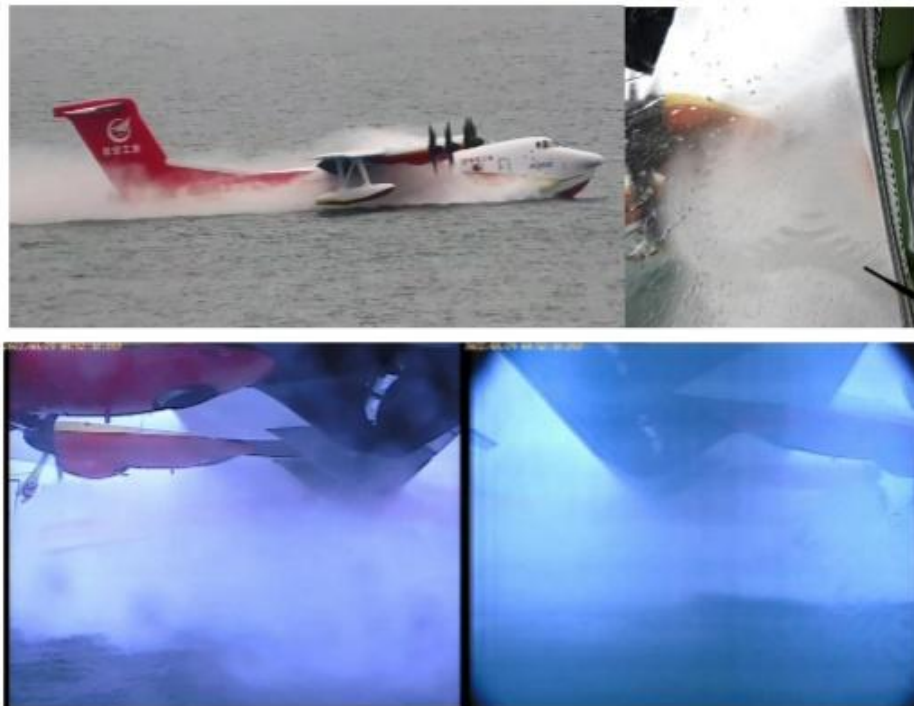
Figure 152: Splash characteristics (take-off)
