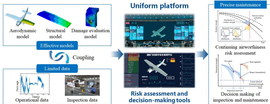
Figure 157: Structural health management of Cessna 172 through the coupling of data and model
