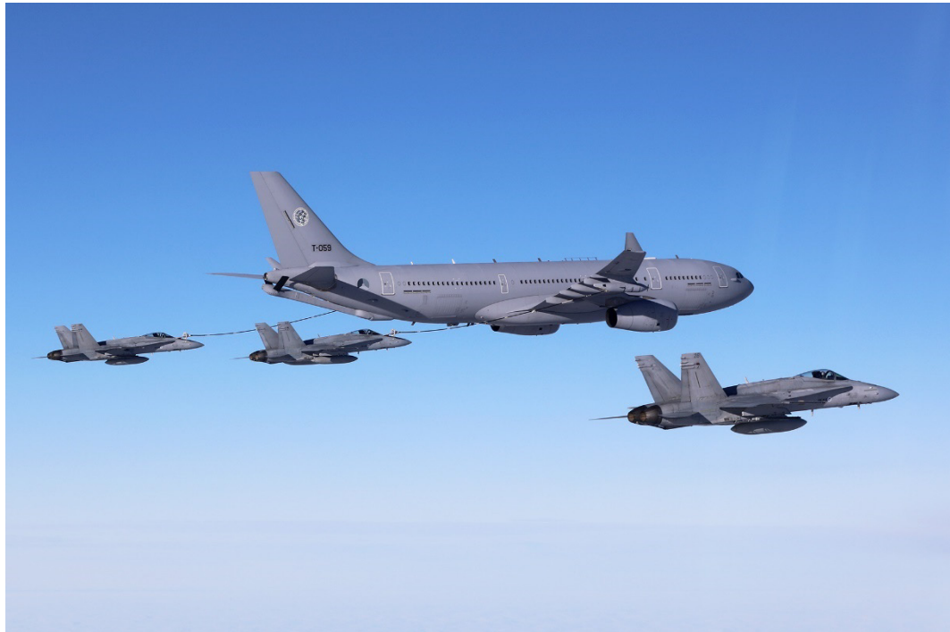
Figure 9: Three FINAF F/A-18C/D Hornet fighter jets (HN-426, HN-456, HN-435) conducting air-to-air (AAR) refueling training missions with the Royal Netherlands Air Force Airbus A330-243 Multi-Role Tanker Transport aircraft (T-059) of the Multinational Multi-Role Tanker Transport Fleet (MMF) in April 2024. Figure courtesy of the FINAF.
