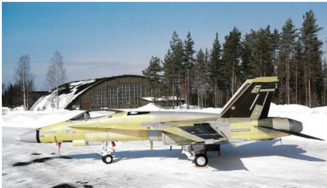
Figure 12: The unofficial rollout view of the first Finnish-assembled F/A-18C Hornet, HN-401, in Halli on April 3, 1996. The material distribution of the yet unpainted aircraft is clearly distinguishable, like the use of composite materials (carbon fiber reinforced plastic) of the structural surfaces. Photo: Jyrki Laukkanen.
