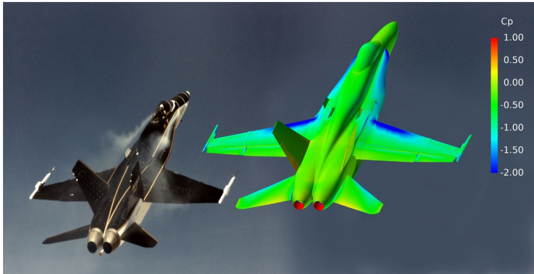
Figure 17: Instantaneous distribution of the pressure coefficient on the aircraft's surface at angle-of-attack = 30 deg and Ma = 0.2755 . Figure courtesy of Elomatic Ltd.
