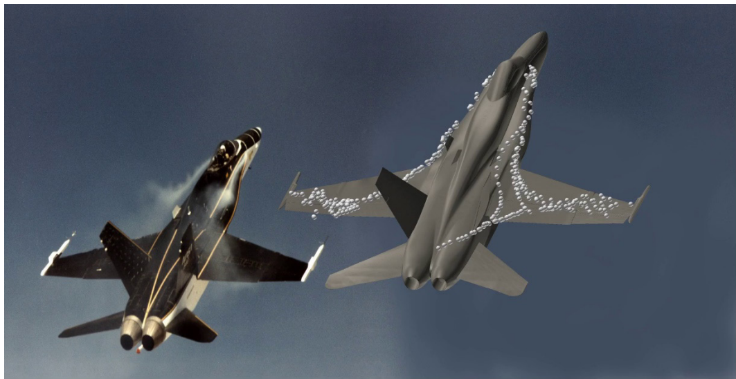
Figure 16: HARV flight test (left) and FINFLO simulation streaklines (right) at constant flight path with \alpha = 30^\circ and Ma = 0.2755 . Figure courtesy of Elomatic Ltd.
