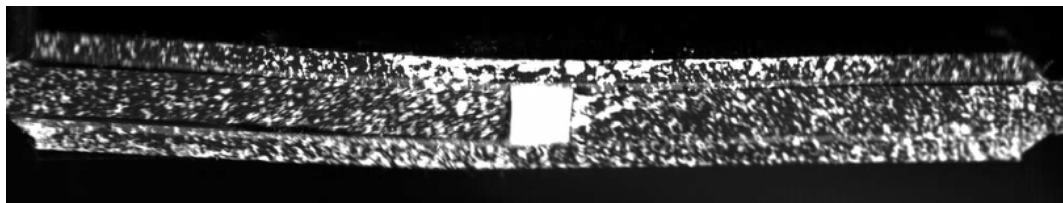
Figure 27: An in-situ image provided for the DIC analysis of the pre-cracked DSJ specimen. [34]
