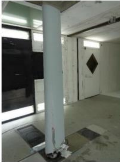
Figure 20. Composite wing located in the wind tunnel and subjected to variable wind speeds and bolt configuration settings
