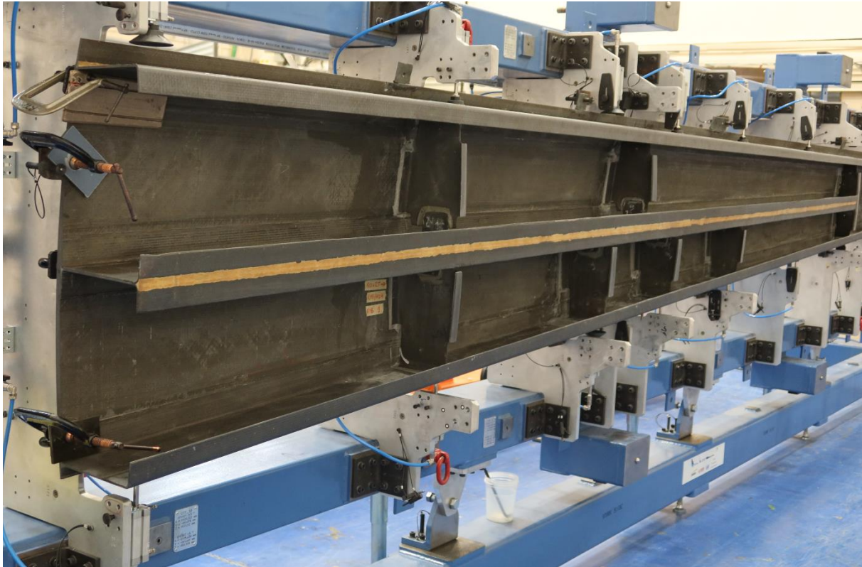
Figure 11. Multi-spar wing demonstrator at the assembly jig before skin attachment
