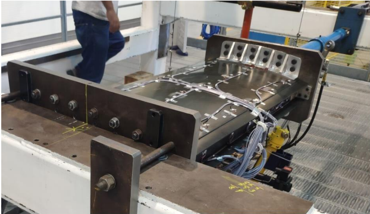
Figure 10. Assembled small scale demo test in Piaggio including optical fibers
