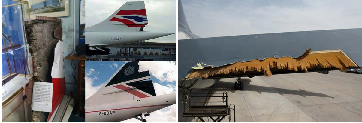
Figure 4.8 Issues related to Hygrothermal ageing: Concorde, 1989 (L); Airbus A310, 2015 (R).
