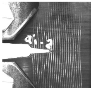
Figure 4.16 Compact Tension/compression experiments to determine intralaminar ERR.
