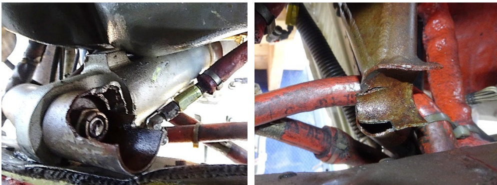
Figure 5.2.2 Fractured portion A (left: actuator side, right: engine mount side)
