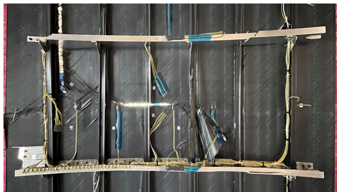
Figure 6 Final failure in tension of the stiffened panel with large notch. Courtesy NLR.
