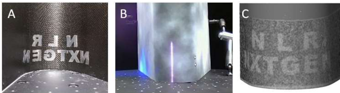
Figure 18 A) The laser ultrasonic scanner. B) A curved CFRP component with markers on the inside. C) The rapid laser ultrasonic inspection. D) The inspection results mapped on a digital representation of the component
