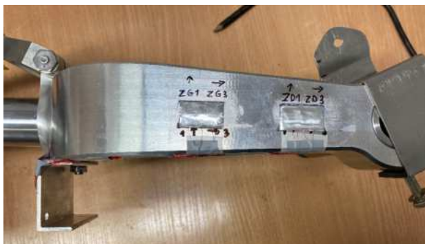
Figure 5.2. Strain gauge placement on NLG half-fork. Source: L-ILot.
