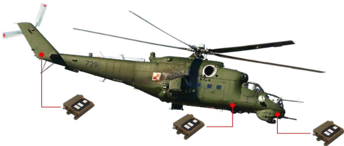
Figure 7.1. CHM system consisting of three autonomous sensors installed on in-service Mi-24
