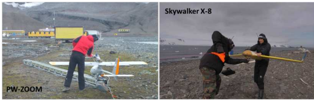
Fig. 1.1. Preparation to the take-off of PW-ZOOM (catapult) and Skywalker X8 (bungee)
