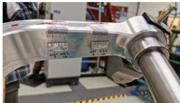
Figure 5.2. Strain gauge placement on NLG half-fork. Source: L-ILot.
