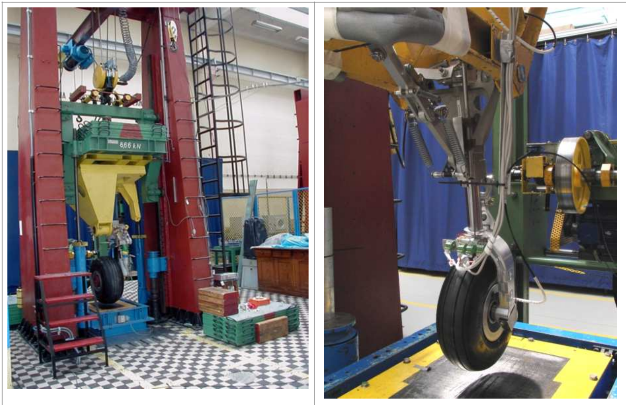
Figure 5.7. M10T test stand – overview example (left), I-31 NLG mounted (right). Source: L-ILot.
