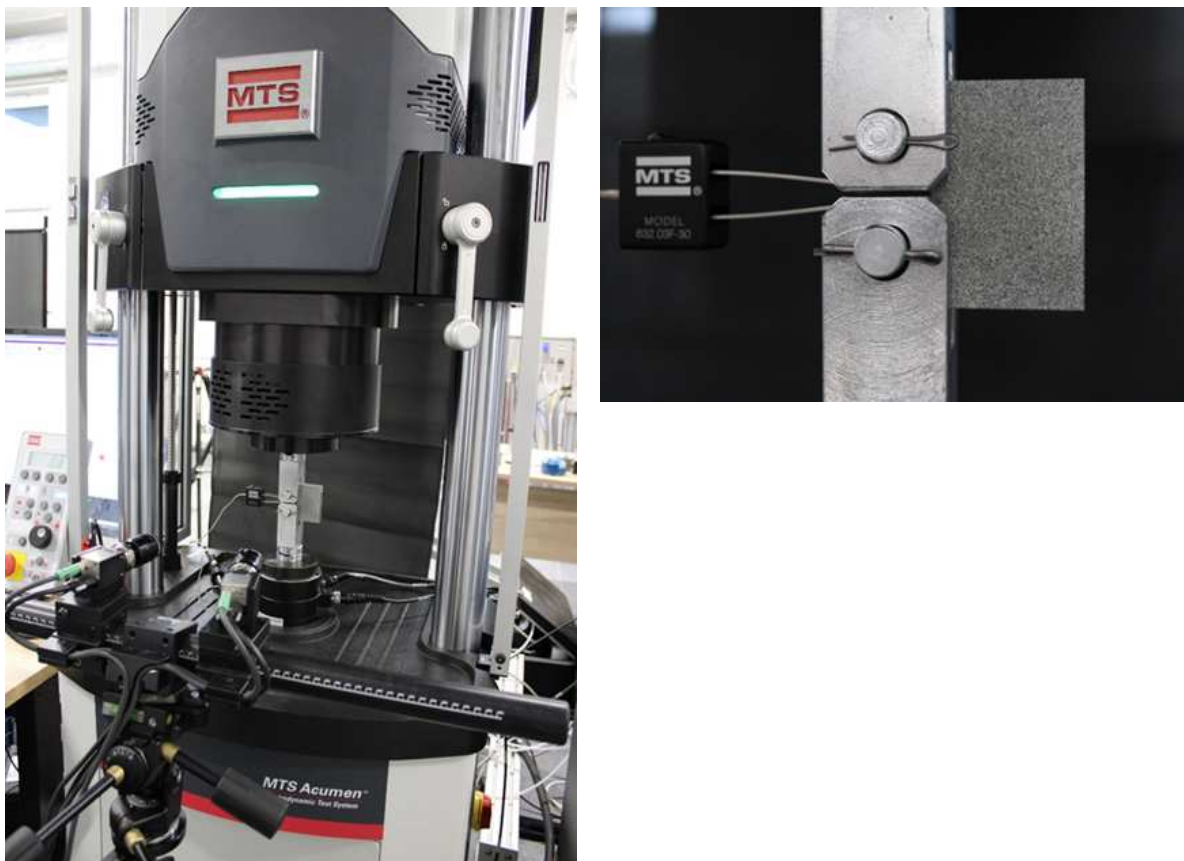
Figure 4.3. Test specimen placed in the test stand. During (with a COD gauge) and after the test
