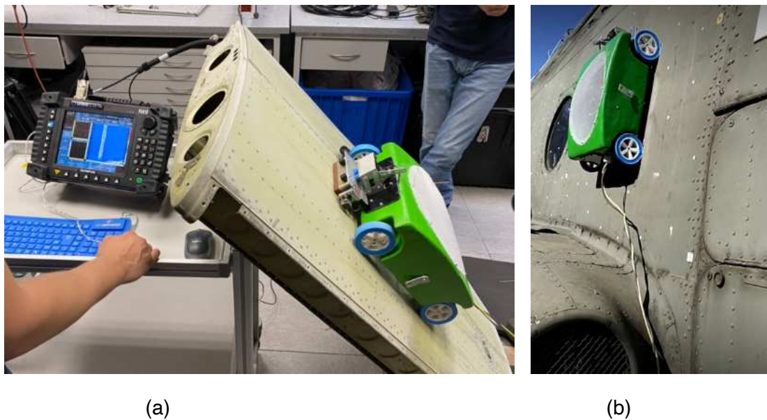
Fig. 2.5. Testing of the developed mobile robotic platform in laboratory conditions and on the fuselage of a military helicopter.
