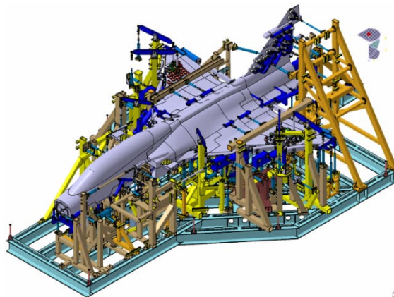
Figure 4.1-5. Full-scale fatigue test set-up, Gripen F airframe.
