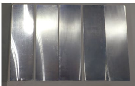
Chromate conversion coating specimens after salt spray 196 hr
