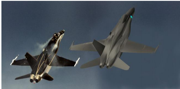
Figure 16: HARV flight test (left) and FINFLO simulation streaklines (right) at constant flight path with \alpha = 30^\circ and Ma = 0.2755 . Figure courtesy of Elomatic Ltd.
