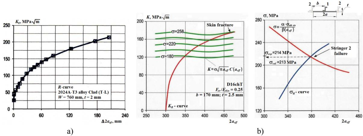
Figure 3. Calculation of stiffened structures residual strength, a) Fuselage skin material R-curve, b) Il-86 aircraft fuselage computed residual strength vs. the experimental one.
