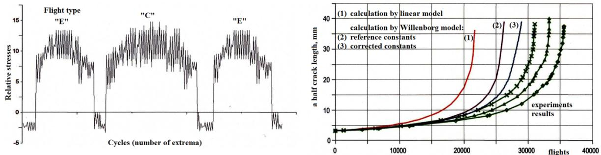
Figure 2. Calculation of fatigue cracks growth rate in aircraft structures.
