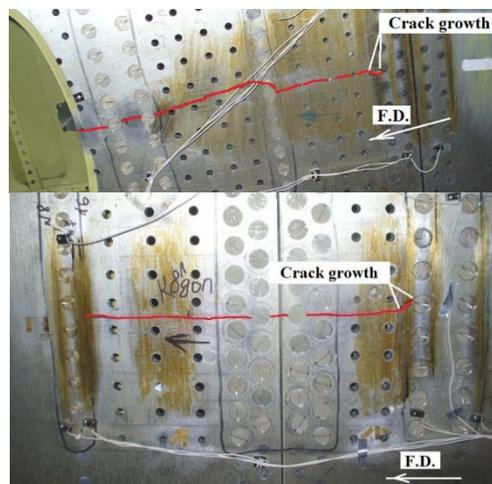
Figure 4. Durability tests of wide-body aircraft wing.
