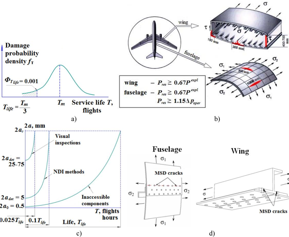
Figure1. Fatigue and durability criteria, a) safe life, b) fail safe, c) damage tolerance, d) prevention of MSD.
