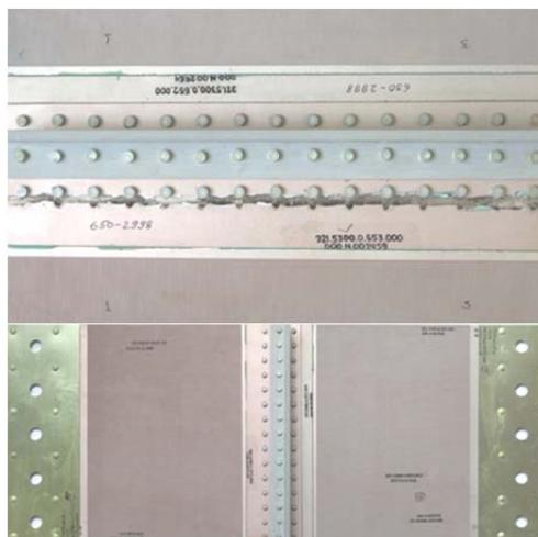
Figure 7. Research of MSD cracks in longitudinal joints specimens of pressurized fuselage skin.
