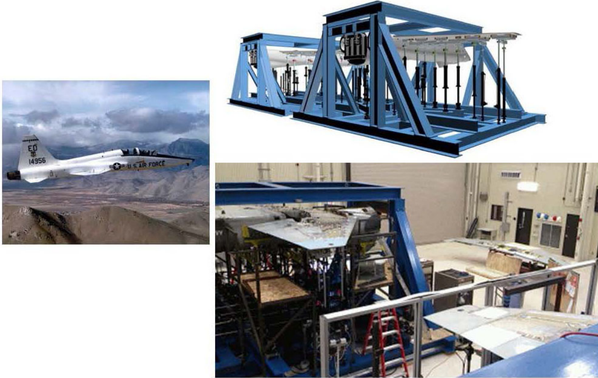
Figure 9.11-89. T-38 Full-Scale-Fatigue Test
