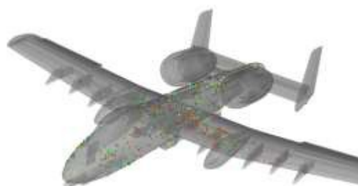
Figure 9.11-74. Test and Teardown Visual Cracking Direction Data
