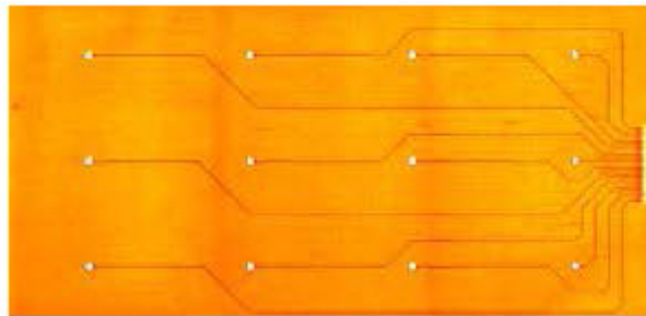
a) Active Damage Detection Sensor
