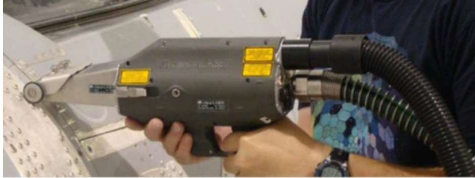
Figure 9.7-15. Hand-Held Laser Paint Removal Tool
