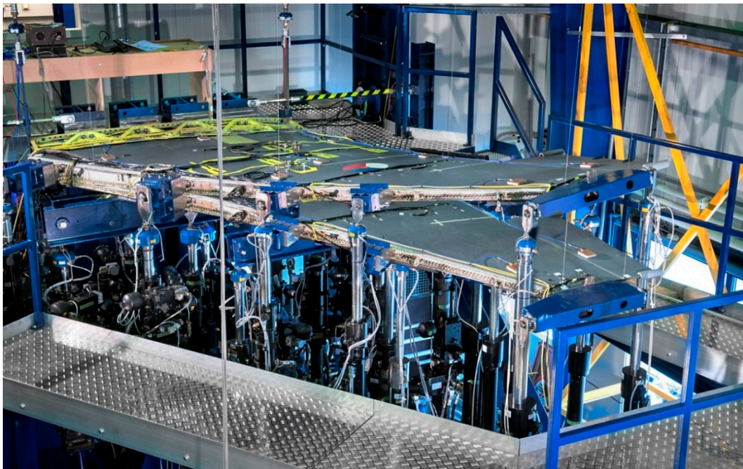
Figure 46: Composite photograph that shows the F-16 Block 15 wing deflections as encountered during the applied limit load cases that represented -3g down bending and +9g up bending.
