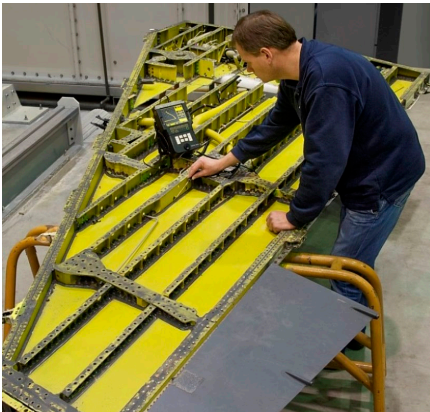
Figure 47: Eddy current inspection of the fatigue critical areas in the F-16 Block 15 left hand side wing during teardown.
