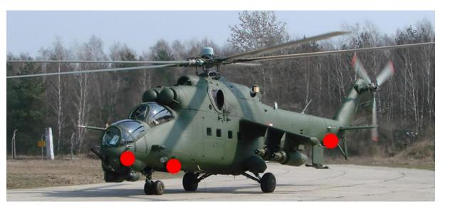
Location of corrosion sensors on the airframe of the Mi-24 helicopter
