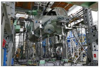
Mi-24 helicopter installed on the test rig
