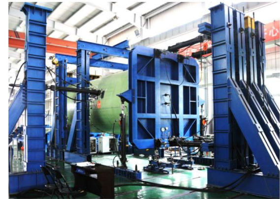
Figure 4-16 The fuselage isometric section test
