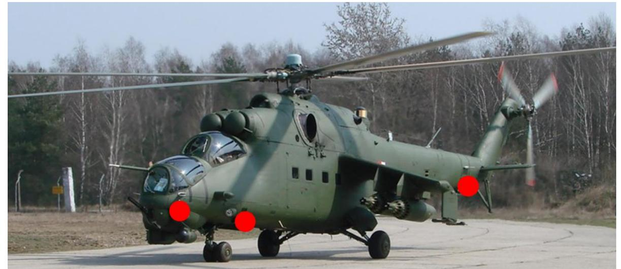
*Location of corrosion sensors on the airframe of the Mi-24 helicopter*
