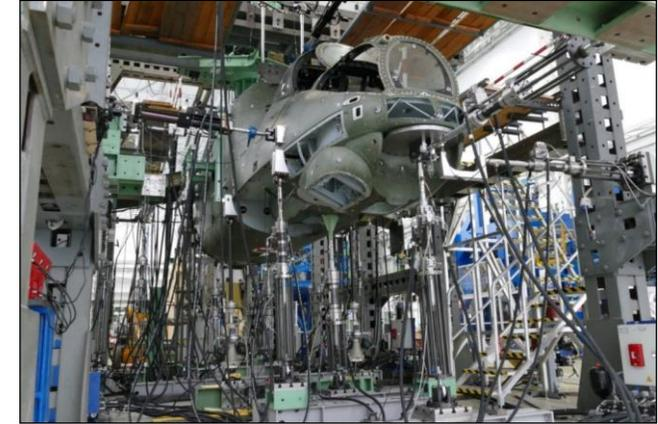
*Mi-24 helicopter installed on the test rig*
