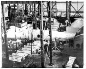
Full scale fatigue test of Yakovlev 40
