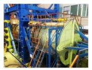
Full scale fatigue test of fuselage section
