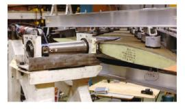
Abt. 800 initial flaws installed in full-scale component testing
