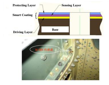
Intellective Coating Monitoring System in Full-Scale Fatigue Test of Aircraft Application of accelerated fatigue life testing in MA600 full-scale test
