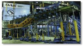
Number of varios configuration wing panels have been tested to be followed by full-scale wing tests
