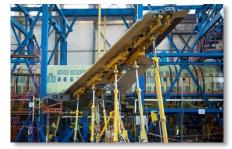
Tests of wing structure to validate SSJ-100 DSO of 60000 flights
