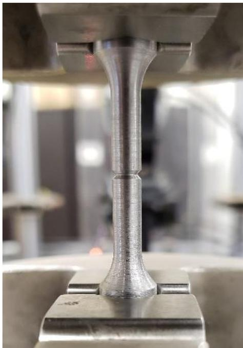
Figure 6: Experimental setup of notched AISI 4340 fatigue coupons.
