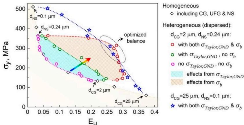
Figure 8: Relation of strength and ductility of heteromaterials with different phases.
