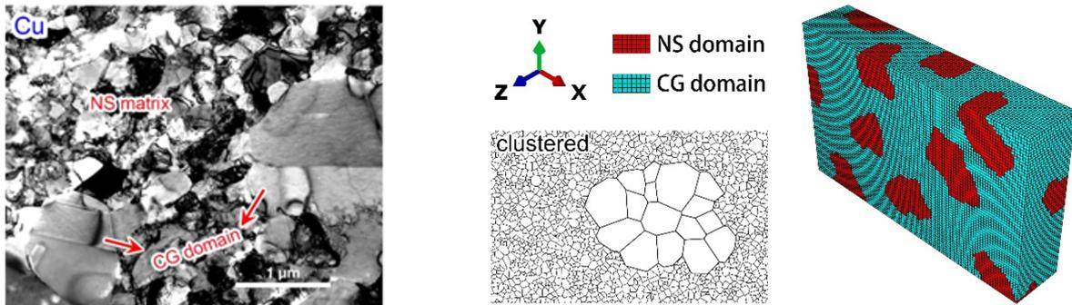
Figure 5: Two-phase metal sample and its finite element model.
