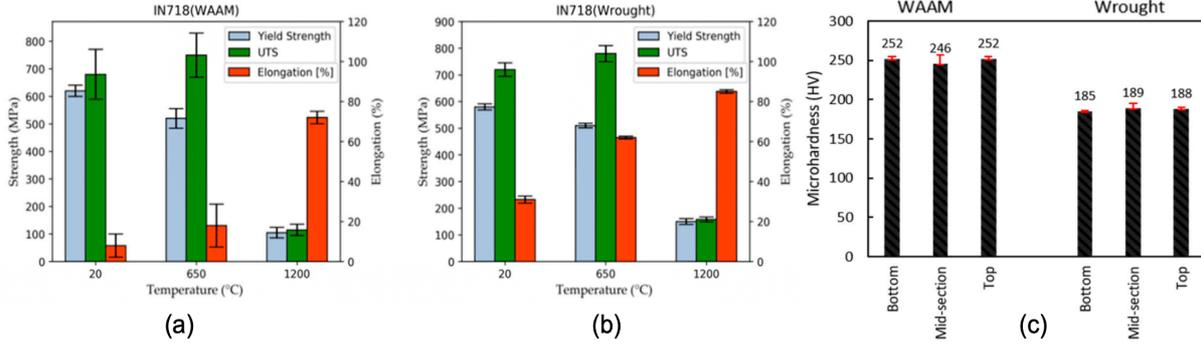
Figure 4: Strength and hardness of WAAM and wrought IN718 alloy in different temperatures and positions in the sample.
