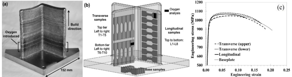
Figure 2: DED fabricated Ti-6Al-4V component and tensile tests from samples of different position and directions.
