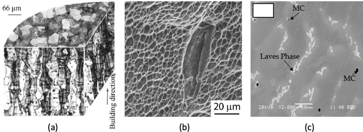
Figure 3: The microscale heterostructures and heterogeneities of AM metal materials.
