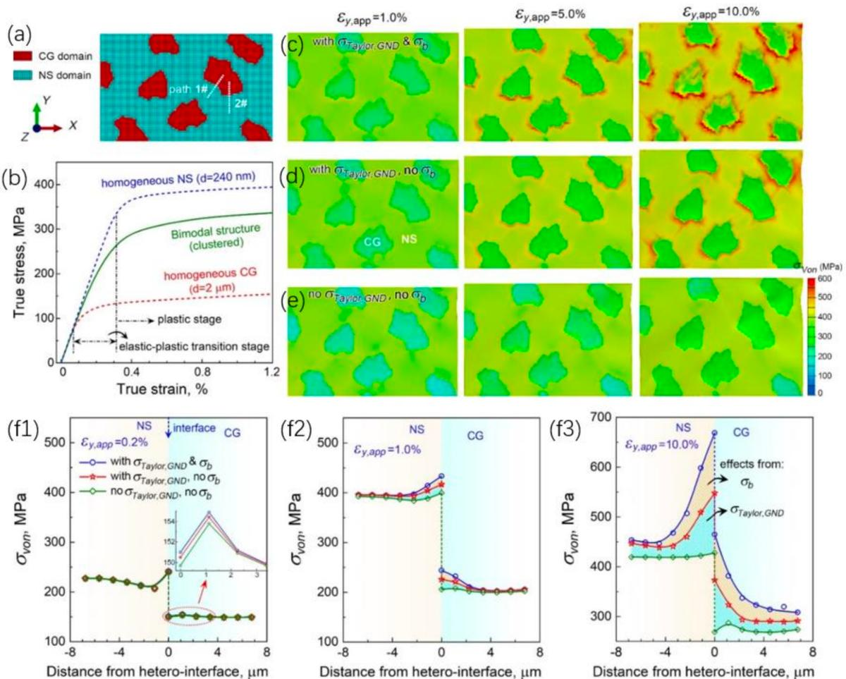
Figure 6: Stress and strain of the heteromaterial and the distribution near the domain boundary.
