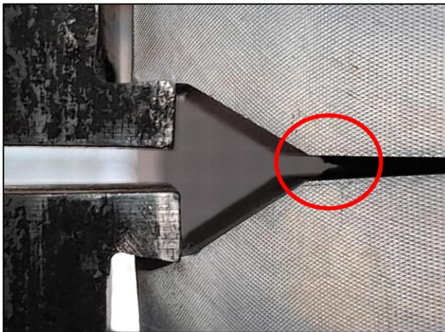
*Chevron specimen with initiated crack*
