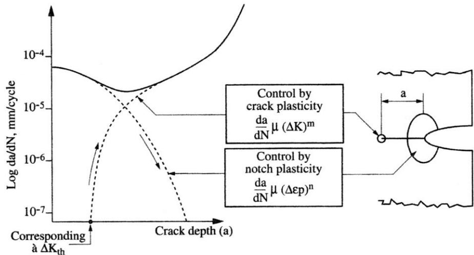
Growth of a short crack affected by notch (Verreman, 2010)
