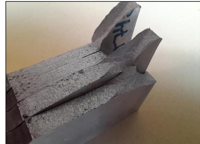
*T7451 and T6I4 fatigue tested C(T) specimens*
