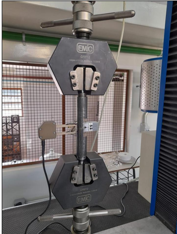
*Chevron-notch fracture toughness test*
