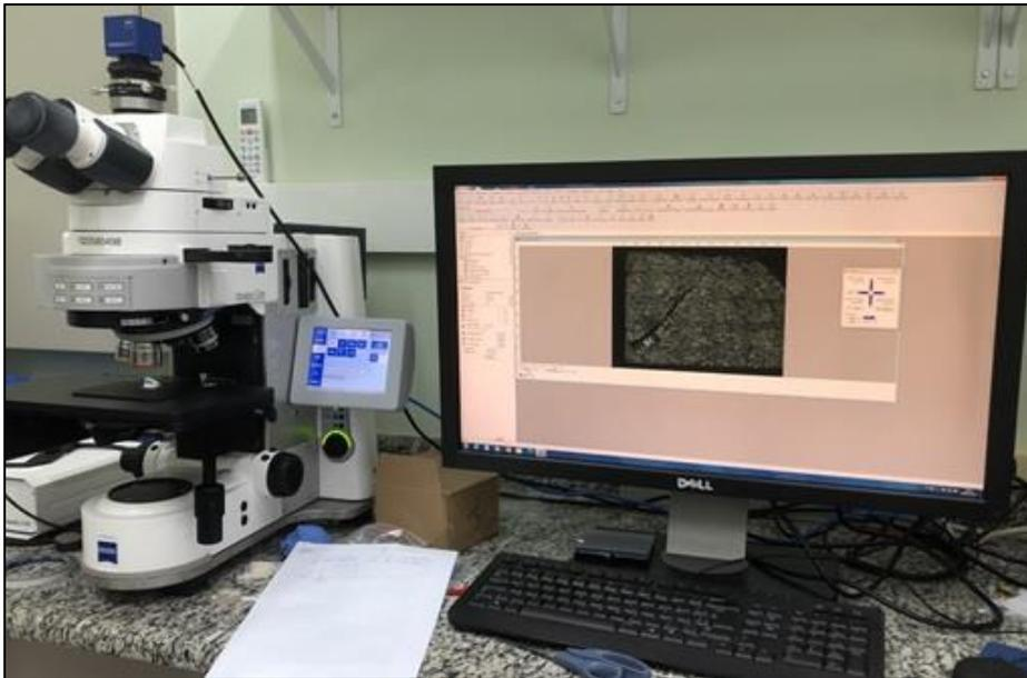
*Zeiss Z2m motorized optical microscope*
