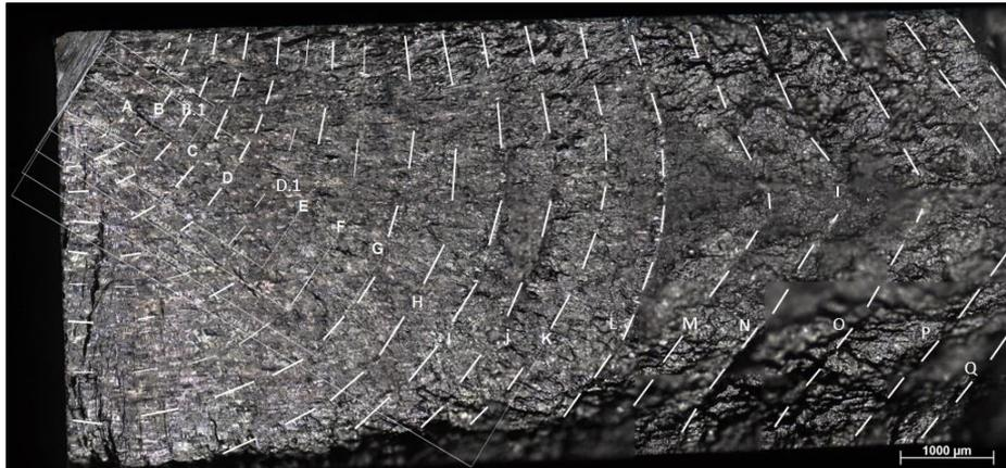
*Fatigue crack growth map, optical micrograph (T7451, 270 MPa)*
