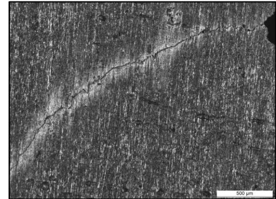
*Crack deviation in T6I4 specimen*
