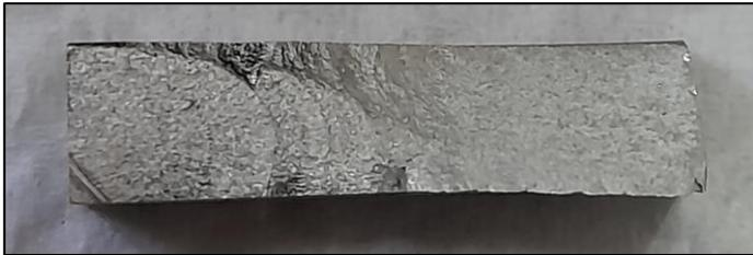
*Spectrum loading fractured specimen (T6I4, 330 MPa)*
