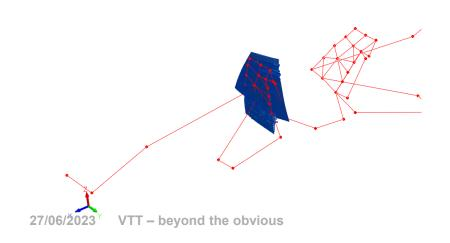
Test Model EMA 8.9Hz vs FEA 14.9Hz (MAC 73.4%)
